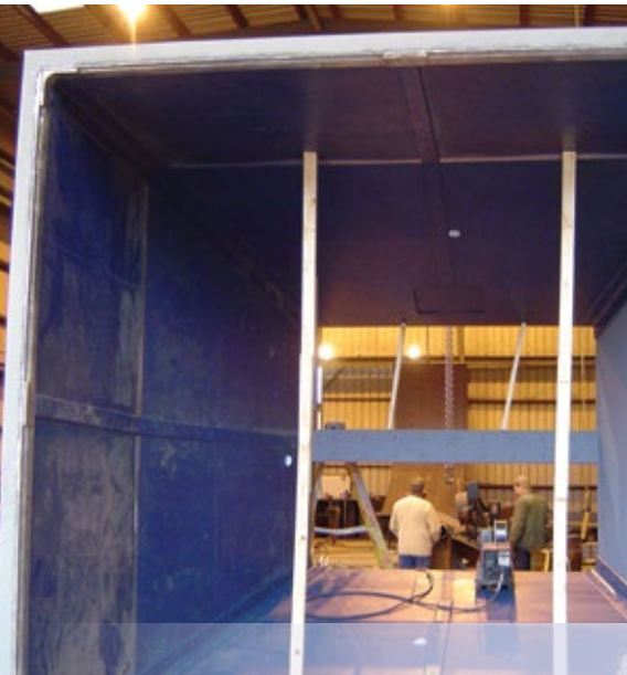
TIVAR® 88-2 lined synthetic gypsum hoppers
