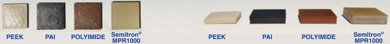
2 KW 03 PLASMA SAMPLES - DISPLAYS MASS LOSS - ALL SAMPLES STARTED AT APPROXIMATELY THE SAME SIZE
